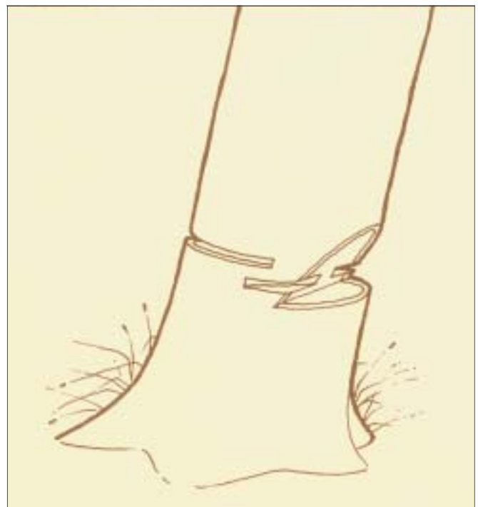
Figure 18. the proper way to cut a tree that is leaning heavily in the correct direction. A cut made in each side on the hinge will prevent the tree from splitting along the grain.
